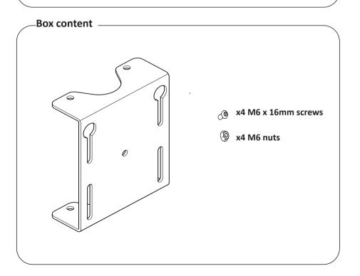
Mount bracket on ceiling pole — 1) M6 x 16mm screws M6 nuts (2) Mount rail on bracket Use nuts and screws from SPDS2116 2 (1) Fix swivel in nuts to the rail  $x4^{\downarrow}$ (2) Fix top screws in to swivel in nuts and slide rail onto the pole
